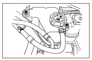
The engine coolant surge tank is located in the rear of the engine compartment.
